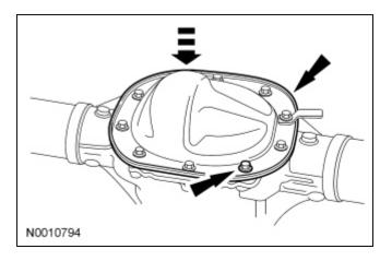
4. NOTE: When filling the axle it must be done on a level surface with the vehicle at ride height.
