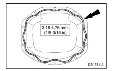
3. **NOTE:** The differential housing cover must be installed within 15 minutes of application of the silicone sealant, or new silicone sealant must be applied. If possible, allow one hour before filling the axle housing with axle lubricant to make sure the silicone sealant has correctly cured.
